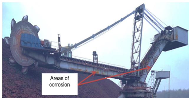
Fig. 1. General view of a machine for extracting coal with corrosion areas the metal structure
